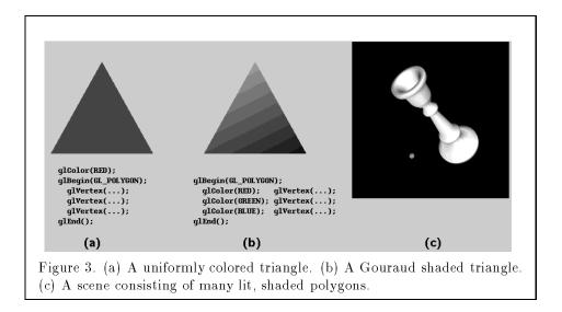
edges described by original vertices; color and texture coordinate values for these new vertices are found by appropriately interpolating the values assigned to the original vertices.
