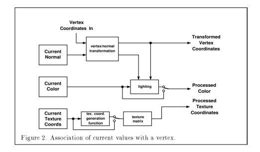
mode) or a single color index value (when initialization specified color index mode). One, two, three, or four texture coordinates determine how a texture image maps onto a primitive.
